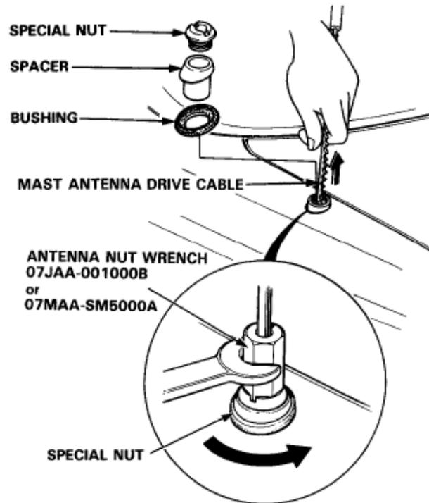
**Step 2.** As someone turns the radio on and as the mast begins or tries to come up, grab hold of it and pull out the old mast. Make sure that the short outer grounding/retaining sleeve has come out with the old antenna mast. This is very important, as this is what holds the antenna mast in when the nut is fastened. If the old mast and grounding/retaining ring are out then proceed with step 4. If not, proceed with step 3.
