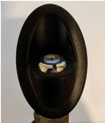
**Step 7.** Thread the new antenna into the adapter and snug it down by turning it clockwise. This should be finger tight but enough so that it's secure. Again, do not overtighten. If the adapter is spinning when threading the antenna, then the nut needs to be tightened more.
